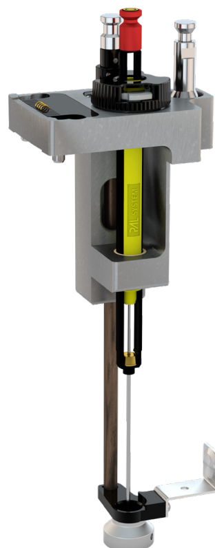
PAL3 Smart SPME Arrow installed in tool.
